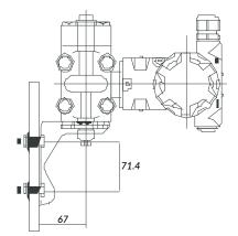
Bending bracket for flat installation
