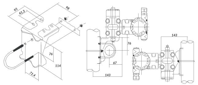
Bending bracket for panel installation
