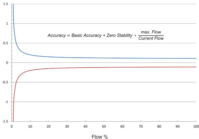
This diagram shows typical values. Individual values may be taken from the calibration records supplied with each meter.
